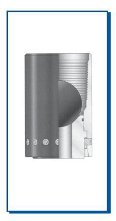
Classic Oilfield's Pump-Out Plug Assembly temporarily plugs the tubing and serves as a temporary bridge plug in the setting of a hydraulic packer. After the production string is landed or the well is prepared for production, the internal plug shears out when appropriate differential pressure is applied to the tubing, leaving a full opening with a wireline re-entry guide shoe on the tailpipe.
