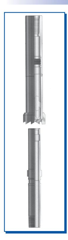
Classic Oilfield's T-2 On-Off Tool enables the tubing string to be disconnected above a packer for zonal isolation, tubing retrieval, and temporary zone abandonment. The tool contains an internal lock profile for landing a wireline plug to provide zonal isolation below the packer.
