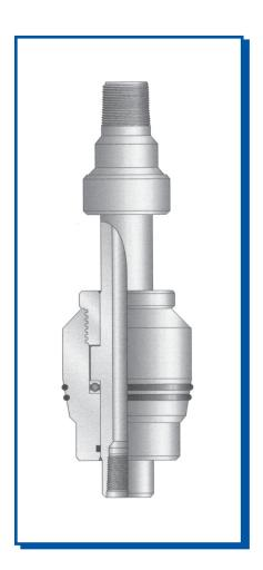
The T Rotating Sub is primarily used in pumping wells which require periodic rotation of the tubing string to prevent extensive wear from sucker rod movement. Rotation of the tubing string can prolong tubing life and reduce expensive workovers. It is also used where a rotational By-Pass Valve is incorporated as part of a completion string. The string can be rotated to open the tubing to the annulus, then rotated again to close the valve.
