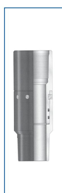
Classic Oilfield's Shear-Out Safety Joint enables the positive release of the tubing string in completions with expected retrieval challenges. The joint is used between packers in single, dual and triple completions. It is also used when rotational release is not wanted.
