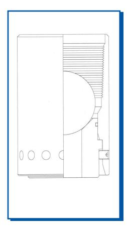
The Classic Oilfield Pump-Out Ball Seat is available with various tubing connections to adapt to tailpipe run below hydraulic set packers. After the production string has been landed, the setting ball is dropped down the tubing. After the ball is on the ball seat, pressure applied to the tubing string will set the packer. Additional pressure will shear out ball seat. With the removal of the plug, the coupling serves as a wireline re-entry guide. Premium threads available upon request.
