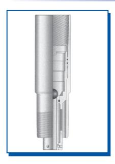
The HLC Hydraulic Landing Collar has an internal ball seat, and is run with Hydraulic Liner Hangers. The HLC Hydraulic Landing Collar is run two or three joints from the shoe, and is used to land the Liner Wiper Plugs. The plugs provide a pressure seal from above and below. The plugs are easily PDC drillable.
