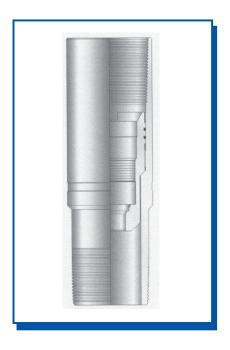
The MPLC Mechanical Plug Landing Collar is run two or three joints from bottom, and is used to land the Liner Wiper Plug. The plugs provide a pressure seal that holds pressure from above and below. The plugs are PDC drillable.
