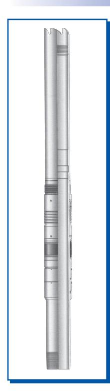
The LLPH Liner Lap Packer, Rotational with hold downs is a versatile liner packer which can be used in an number of different applications. It is most often placed at the top of a liner which is to be cemented. Setting the type LLPH Packer after cementing allows the operator to reverse excess cement out of the hole without exerting pressure on formations below the top of the liner.
