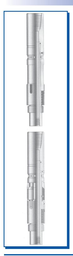
The MLRT Mechanical Liner Running Tool is used to run and set liner into the well bore. It is used to set left hand mechanical liner hangers and hydraulic liner systems. Right hand rotation releases the tool from the liner and is retrieved with the drill pipe at the end of the cementing, or dropping off of the liner.
