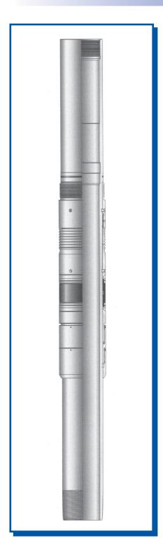
The LLPH-NR Liner Lap Packer, Non-Rotational with hold downs is a versatile liner packer which can be used in a number of different applications. It is most often placed at the top of a liner which is to be cemented. Setting the type LLPH-NR Packer after cementing allows the operator to reverse excess cement out of the hole without exerting pressure of formations below the top of the liner.
