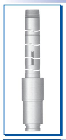
The RPOB Pack-Off Bushing is made up with the liner setting tool using a Cementing Seal Joint polished nipple to extend down through its I.D. A profile to receive and hold the bushing in place is machined into the I.D. of the setting collar, or the packer. After cementing, the Cementing Seal Joint and bushing is retrieved with the setting tool.
