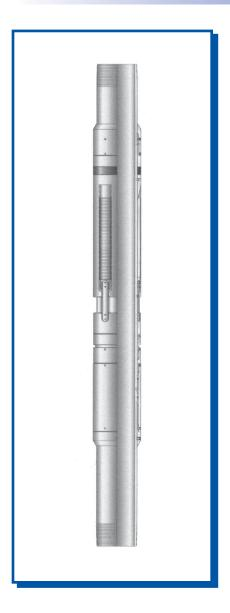
The Hydraulic Dovetail Liner Hanger is a premium hanger with an integral body. The hanger mandrel is machined from heavy wall mechanical tubing and treated to the required grade. Integral construction eliminates all internal connections which provide maximum pressure ratings and liner hanging capacity.
