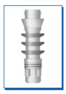
The LWP Liner Wiper Plug with Rotation Prevention Clutch on the nose of the plug lands and locks in place in the seat of the landing collar. Both the Pump Down Plug and the Liner Wiper Plug act to hold pressure from above and below.
