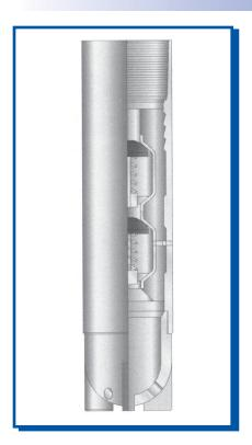
The Double Valve Float Shoe, Spaded Nose, features back pressure valves and a spaded nose with circulating side ports. The side ports are used when liners are set on bottom, this improves cementing operations. The Double Valve Float Shoe, Spaded Nose is PDC drillable.
