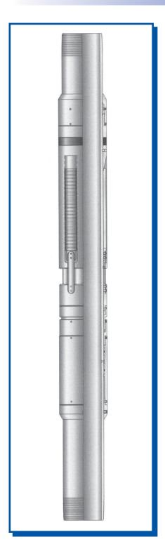
The Hydraulic Dovetail Rotating Liner Hanger is a premium hanger with an integral body. The hanger mandrel is machined from heavy wall mechanical tubing and treated to the required grade. Integral construction eliminates all internal connections which provide maximum pressure ratings and liner hanging capacity. This premium liner hanger can be rotated into place, set and then rotated through the liner cementing operation.
