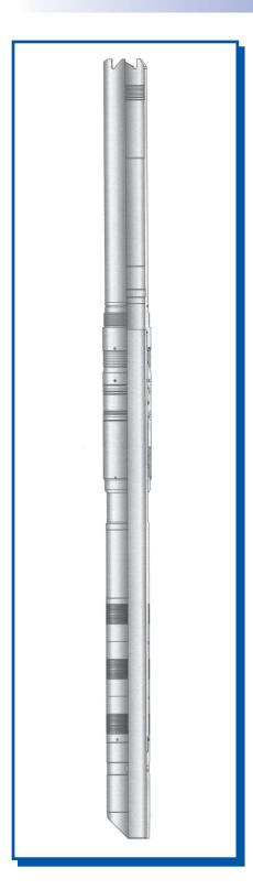
The LTBPR Liner Tie-Back Packer is a high-pressure seal at the top of a cemented or uncemented liner. It is run on drill pipe and / or casing, and landed in a receptacle at the top of the liner. In most applications a type Tie-Back Receptacle is run with the packer providing for future tie-back.
