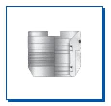
The Drillable Pack-Off Bushing is a high pressure, high temperature pack-off used when working with high angle well bores. The DPOB has Chevron-type packing that seal tightly around the polished stinger of the MR setting tool. The DPB holds pressure from above and below, and is not damaged from rotation during setting or releasing of liners.
