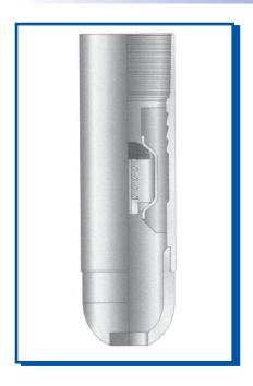
The Single Valve Float Shoe, Spaded Nose, features a back pressure valve and a spaded nose with circulating side ports. The side ports are used when liners are set on bottom, this improves cementing operations. The Single Valve Float Shoe, Spaded Nose is PDC drillable.
