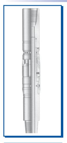
The Rotating Setting Dog is used whenever compressions set liner packers are run. The dogs are spring loaded in the collapsed position while the liner is being run and cemented. When released from the setting sleeve, set down weight is applied to compress the liner packer. Bearing race in the RSD tool is used to transfer additional weight in high angle well bores.
