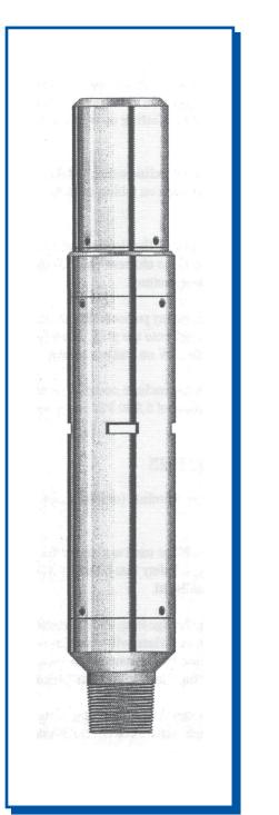
The By-Pass Valve is a rotational circulating valve designed for use with the SST Tool. This valve opens or closes off communication between the tubing and the annulus.
