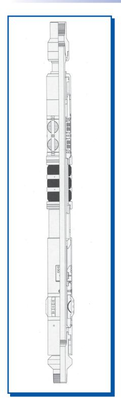
The Classic Oilfield's CST Packer is a three-quarter-turn, compression-set, retrievable service packer capable of holding differential pressure from above or below. The CST packer can be used for conventional service work such as acidizing, fracturing, squeeze cementing and casing tests.
