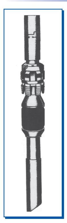
The Classic Oilfield CAD-1 is a tension set, single grip, retrievable debris hold down packer. The CAD-1 is compact, inexpensive and commonly utilized for circulating down wiper plug floating in well bore or holding down undesired debris in well bore.
