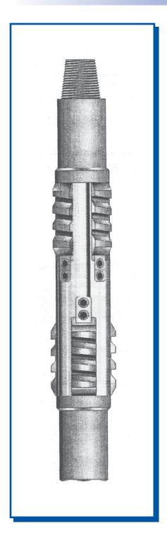
The Classic Oilfield Casing Scraper is used to remove foreign matter on the inside casing wall in order to provide a smooth clean casing I.D. for running and setting packers and other sub-surface equipment.
