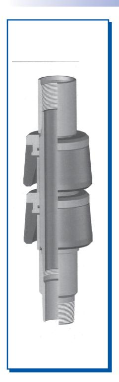
The Classic Oilfield Type GV Cup Packer is an economical means of isolating casing leaks and depleted zones and is also a production or injection packer for low pressure applications. Depending on application, this packer can be run with cups opposed or in the same direction. The GV Cup Packer is also available with packing element back-up rings for higher pressure applications and comes in a full range of tubing and casing sizes in two-cup or four-cup models.
